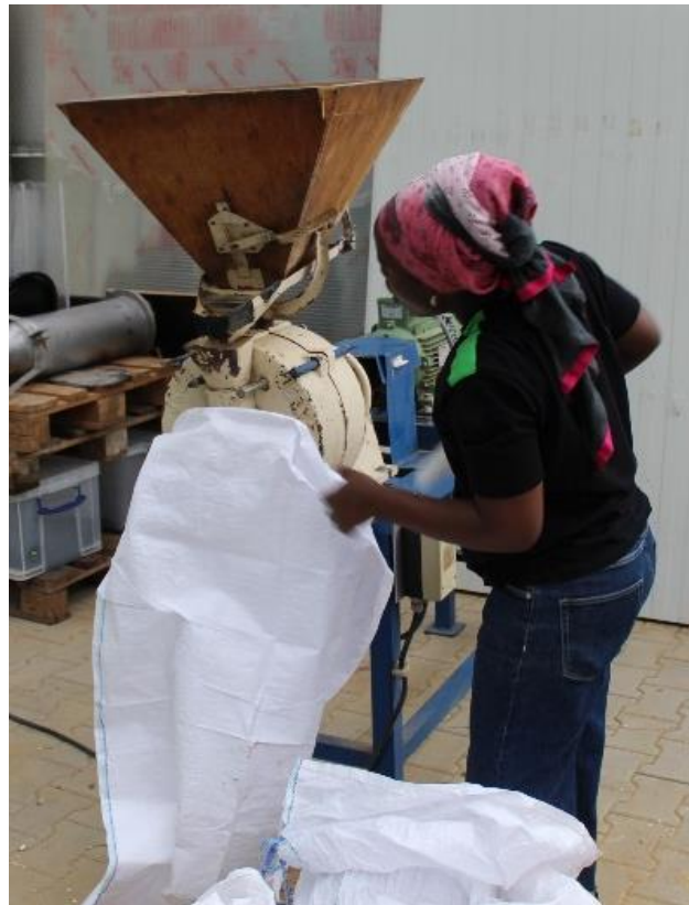
Crushing of biomass to determine energy content, Picture credit: 440e
