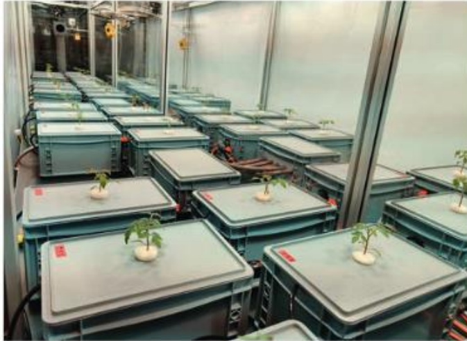
Test setup to investigate the optimum growth conditions depending on nutrient solution salt concentration levels at the Hohenheim University Phytotechnical Center
