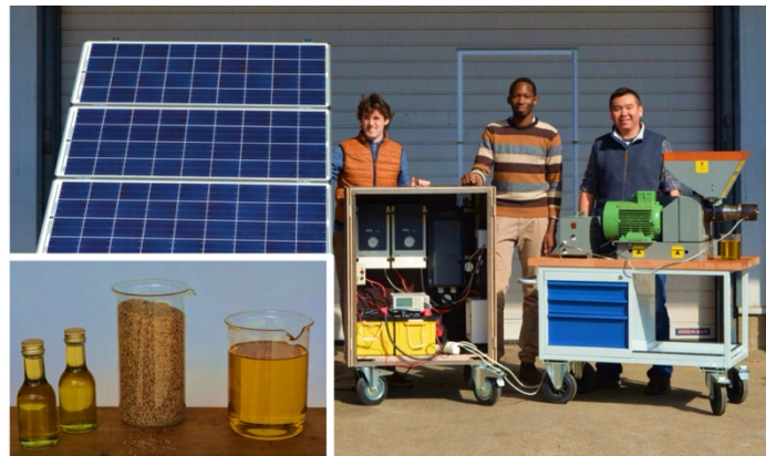
PV-system for solar oil extraction, Picture credit: 440e
